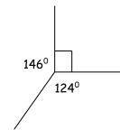
$146^{\circ} + 90^{\circ} + 124^{\circ} = 360^{\circ}$
